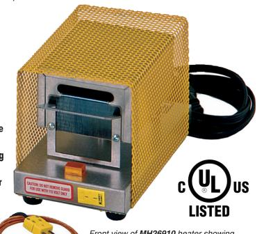
Front view of **MH26910** heater showing inspection kit, which includes Type K thermometer connector wire and screw bit to open rear tamper-proof cover plate.
