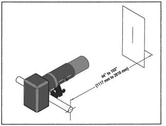
**To Focus:** Loosen nut on outer tube of projector and slide the tube in and out until the line is sharp, then retighten nut. **To Adjust:** Use fingertip adjustment on mounting bracket -- allows line adjustment in all planes.
