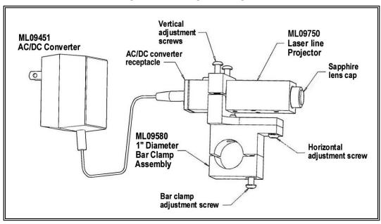
The Everhard ML09750 laser line projector is a Class II laser product. This laser product has a maximum power of 1 milliwatt or less. The unit is considered "eye safe" under normal operating conditions.
