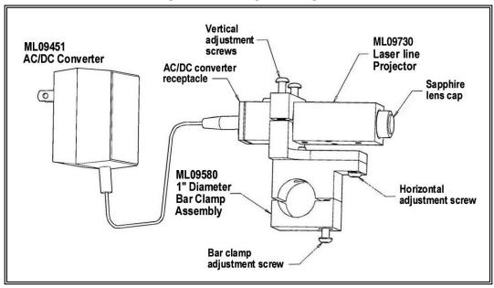
The Everhard ML09730 laser line projector is a Class II laser product. This laser product has a maximum power of 1 milliwatt or less. The unit is considered "eye safe" under normal operating conditions.
